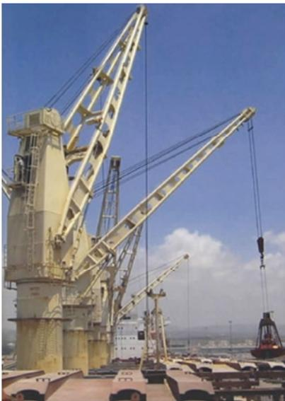
Figure 1 - Luffing jib deck cranes
