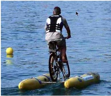
The stock answer to this question is ‘a ship floats because it displaces its own weight in water’. It is true that a floating ship, dinghy or pedalo, does displace a mass of water equivalent to its own weight and all the cargo, kids, beer cans – and bikes – it might happen to carry. But this oft recited fact masks a deeper and more interesting reason for a ship either floating or not floating.
