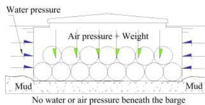
Atmospheric pressure equates to about 1Bar ( $10^5 \text{ N/m}^2$ ). Therefore, every square metre of the barge flat bottom was subject to an atmospheric force of about 10.2ton. As the barge measured about 30 x 11m the total weight of air pressing it onto the mud was almost 3,400tons. By comparison, the fully loaded displacement of the craft was only about 1,000ton.
