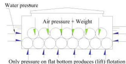
Archimedes only applies to freely floating bodies. While it offers a convenient and reliable means of relating the weight of a ship to its draught it needs to be fully understood if errors are not to occur.
